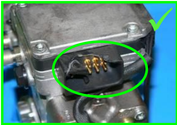
broken connector → acceptable
