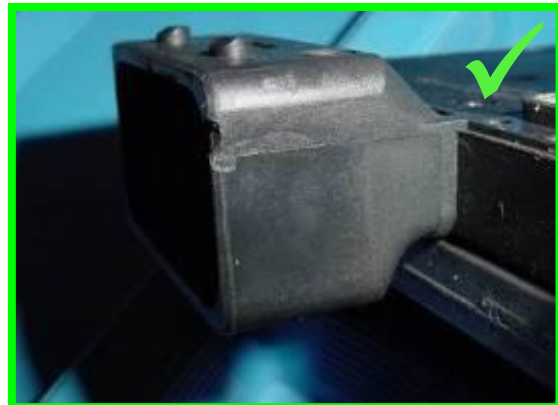
Slightly damaged connector max 2mm → acceptable
