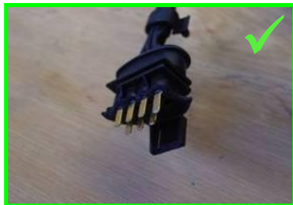
Defective circuit points → acceptable
