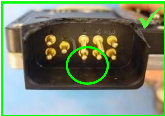
Damaged pins → acceptable
