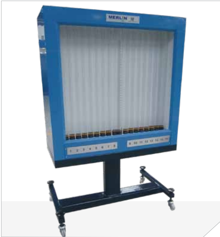
Examples of special production calibrating and injector mounting units R418/3 and C418-3 consisting of 18 x 1000cc and 3 x 3600cc graduates and 18 S or T injector mounts plus 3 x engine injector mounts.
