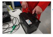
Connect the supply connectors to the battery Red to the battery +ve and black to the –ve/0V).
