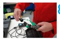
Connect the adaptor cable to the injector
