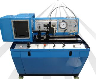
A variable pumping rate allows for critical analysis of nozzle spray form and line pressure can be held to enable stable pressure dry seat testing.
